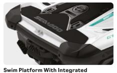
**LinQ System**Exclusive quick-attach system on a large swim platform that allows for easy installation of accessories.
