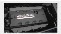
Supercharged, DOHC, 16V 1,812cc engine
